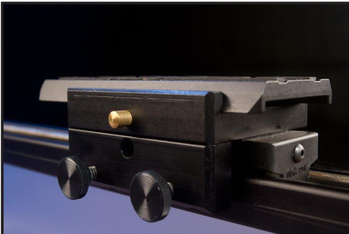
To operate the Dovetail Quick Release plate, first you must locate the lock knob on the side of Quick Release Adapter. (See *figure 29*)
