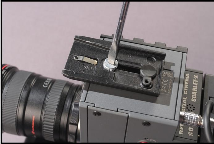
After lining up the Dovetail Quick Release Plate to the thread inserts on the bottom of the camera, use a 1/4-11 or 3/8-11 screw to attach the plate to the camera. (See **figure 23**)
