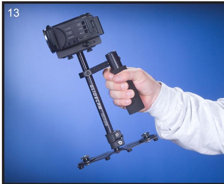
The best way of adjusting the horizontal balance is to move the center of gravity of the camera. This can be accomplished by either repositioning the camera on the HEAD PLATE, or by adjusting the position of the HEAD PLATE, either front to back or side to side with the camera on it.
