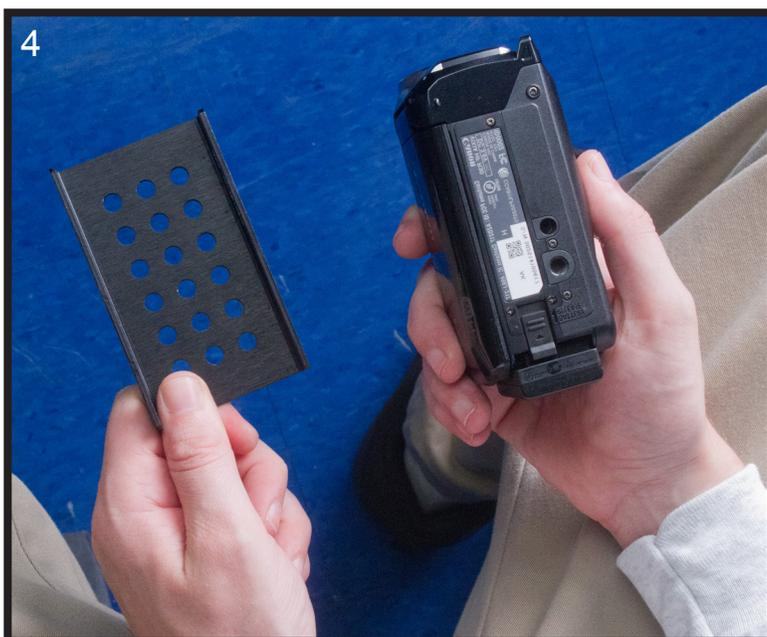
Remove the HEAD PLATE from the Glidecam iGlide and with the camera placed upside down in your lap align the appropriate hole in the HEAD PLATE with the threaded insert in the bottom of the camera. As shown in photo # 5.
