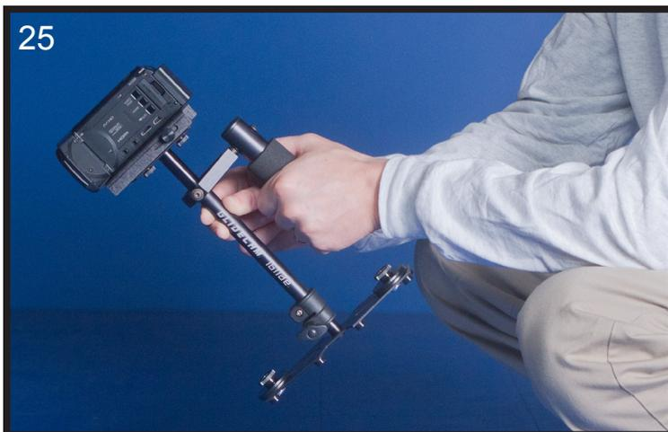
Operating the Glidecam iGlide for extended periods of time can easily tire your holding hand. If fatigue sets in while shooting you can try operating the Glidecam iGlide with your other hand. You can also rest for a while by placing the unit on the ground, or by holding the unit with your guiding hand.
